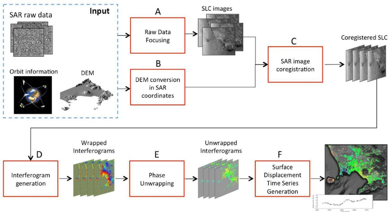
**Simplified block diagram of the P-SBAS processing chain**
