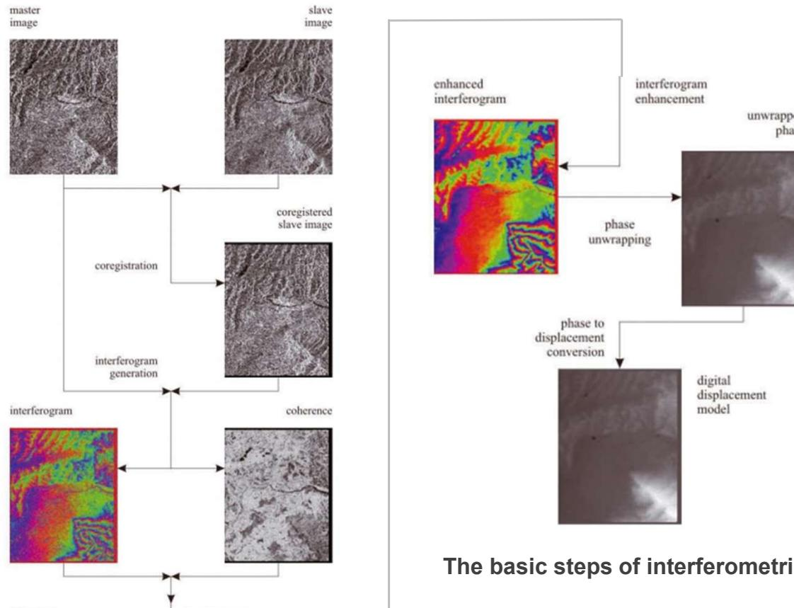
The basic steps of interferometric processing
