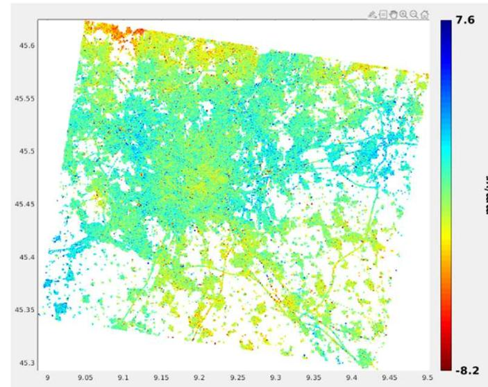
Velocity map with total DEM error, ramps estimation
