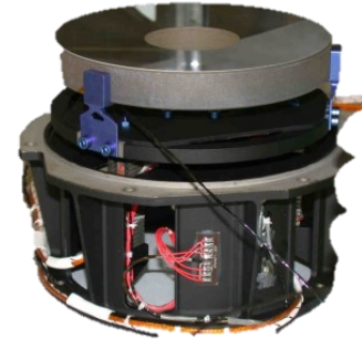
[SODISM Pointing Mechanism, from Meftah, et. Al., 2011]
