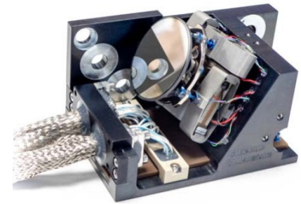
[Point Ahead Mechanism (PAM), from Guignabert, et. Al., 2020]
