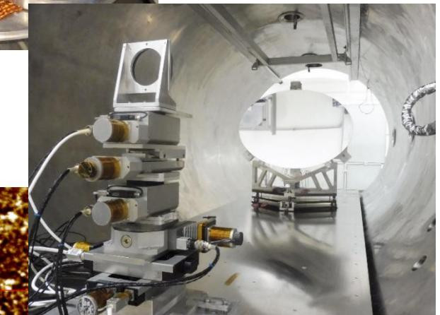
Loading of the PTM in a cryochamber for testing
