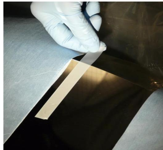
*Adhesion test on the M1 Demonstrator (Credit: MediaLario)*
