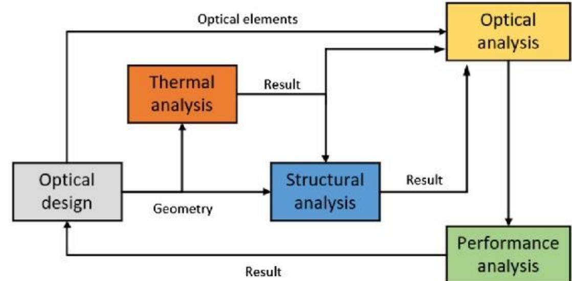
*Diagram of STOP Analysis process flow*
