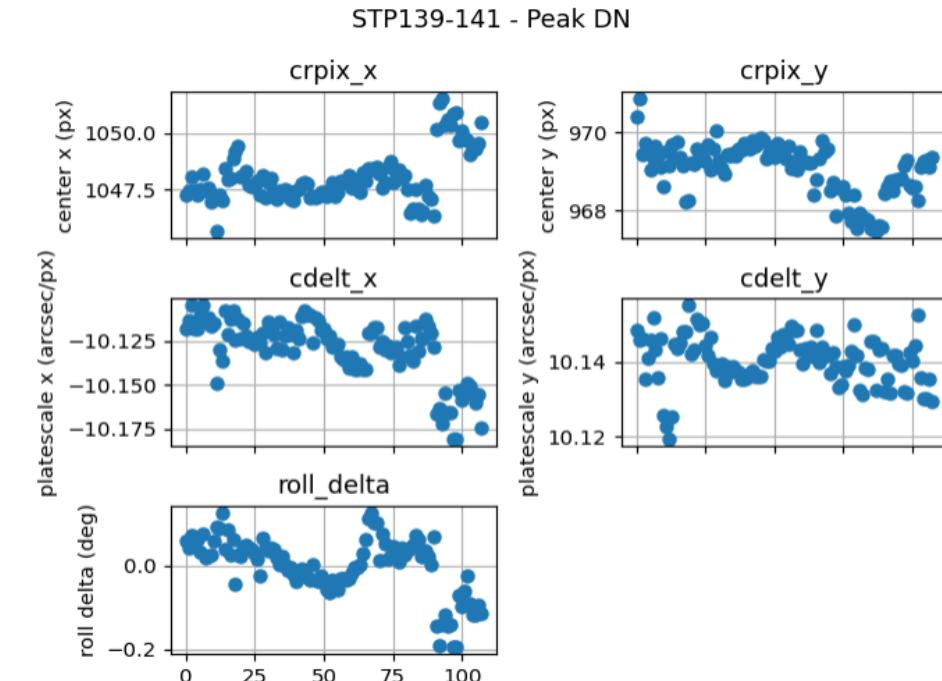
Geometric calibration parameters for a series of Metis Images
