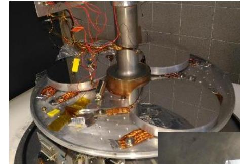
150 mm samples being loaded in a cryochamber
