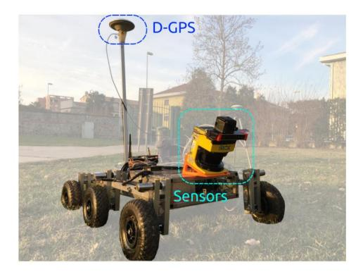
Tested with our MORPHEUS mobile robotic platform instead of an UAV -> LiDAR is 5kg!
