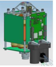
NASA Mars Helicopter Scout, sensor assembly. Monocular vision setup (2° camera only for sporadic hi-res images, not used for navigation) [1]
