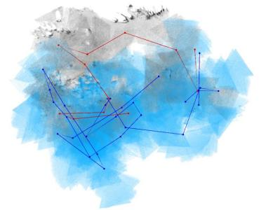
Automatically merged maps from the LRU (Lightweight Rover Unit) and LRU2 rovers on Mount Etna
