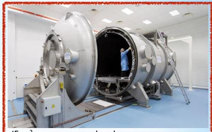
45 m<sup>3</sup> cryo-vacuum chamber 77K and 10<sup>-6</sup> mbar Large integration room (100tn seismic mass to provide high stability (< 10<sup>-7</sup>g at 5 - 100 Hz))
