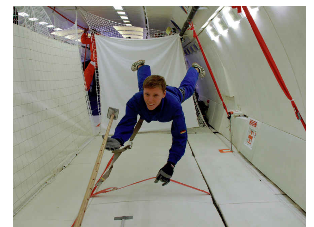
Boom deployment test during parabola flight
