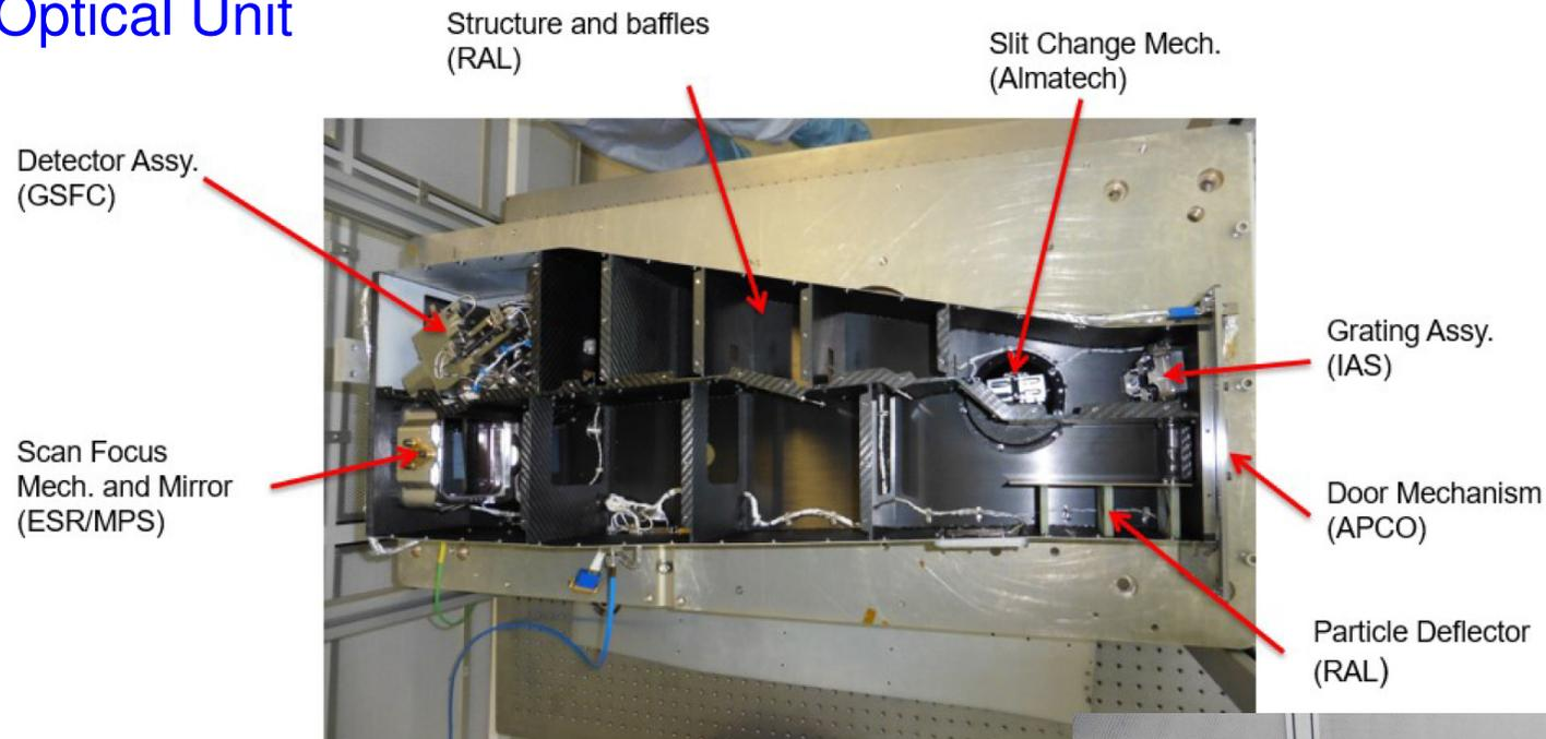
Single-mirror *telescope* with  $f=622$  mm (off axis paraboloid operating at near normal incidence).
