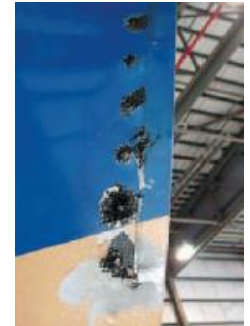
Damage caused by a lightning strike on an aircraft rudder.
