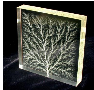
Dielectric breakdown in a solid insulator.
