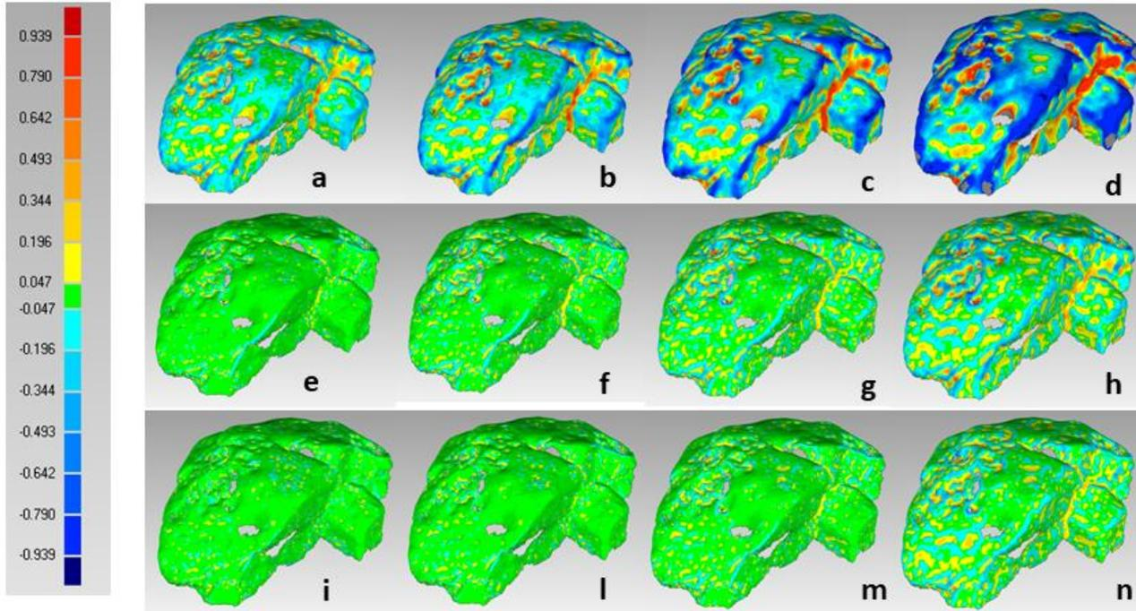
Map of deviation between the raw cloud and the cloud with the application of the smoothing algorithms.
