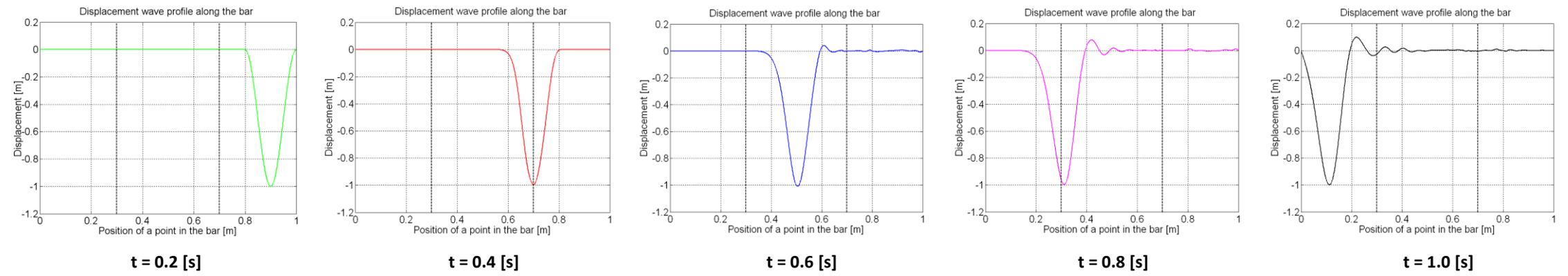
Example of wave propagation and perturbations in a 1D system discretized using (a) FEM and (b) PD. In the example,  $E=1$ ,  $\rho=1$ ,  $A=1$ ,  $\delta=0.031$ ,  $\lambda=0.2$ , and  $\delta/\lambda = 0.155$  in consistent units
