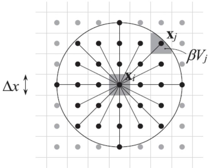
**Representation of a generic horizon in a discretized form.  $\Delta x$  is the grid spacing of the discretized model.  $m = \delta/\Delta x = 3$  in the figure**
