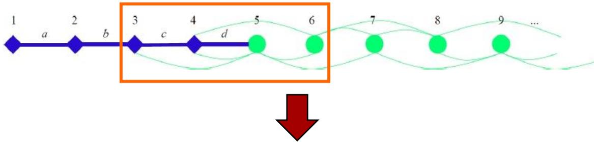
A **coupling zone** is defined where **forces** are **exchanged** between the **FEM** and **PD** parts of the domain
