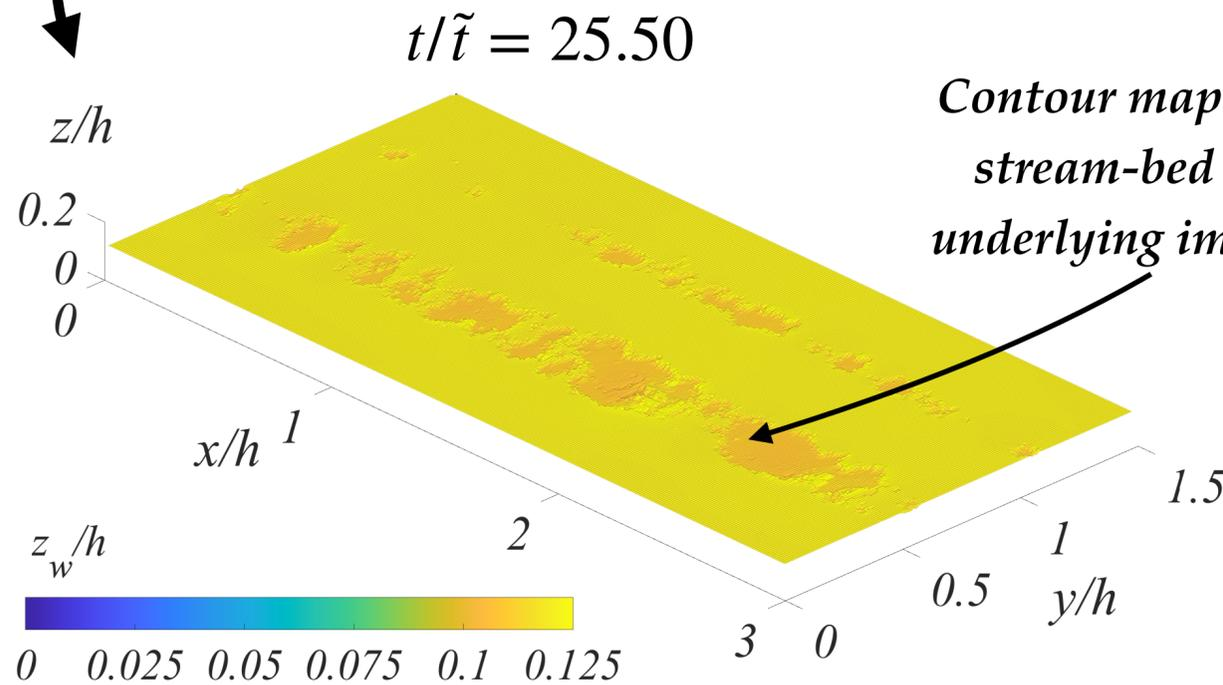
*Contour maps of the height of the stream-bed measured from the underlying impermeable substrate*
