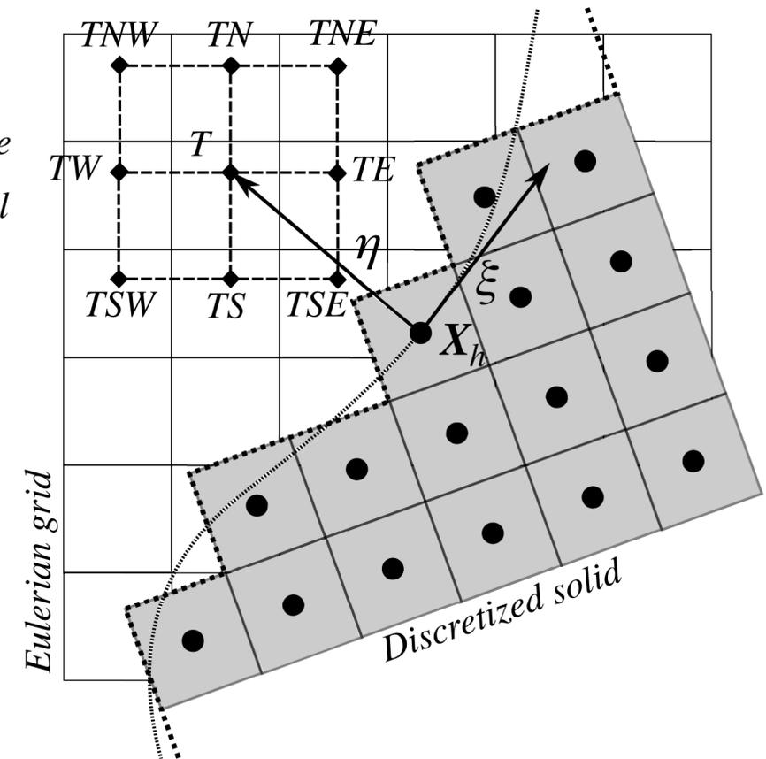
2D schematic of the interpolation stencil used to compute shear and normal stresses in the local frame of reference
