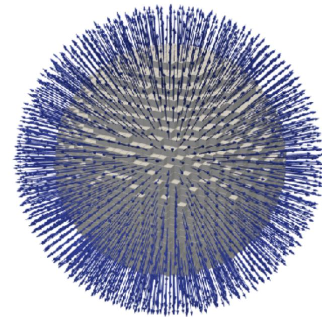
Normals computed on the surface of a peridynamic-discretized sphere
