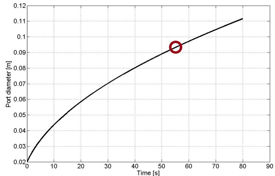
It was demonstrated that at first approximation there is a **linear relation between the regression rate multiplied by the burning time and the size of the motor** in order to keep a fixed shape of the fuel grain
