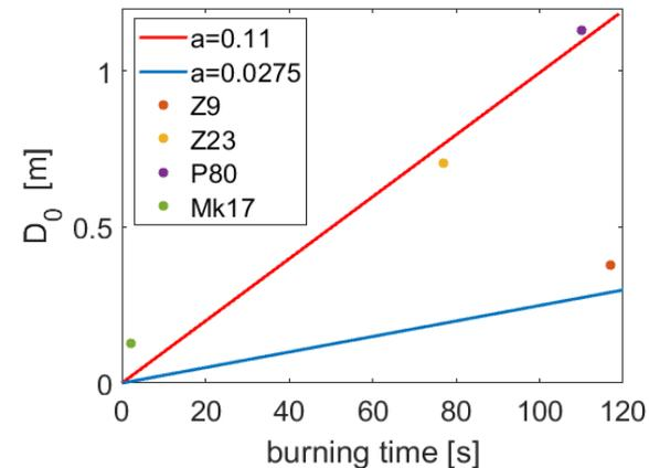
High regression rate is needed for large motors and high volume loading
