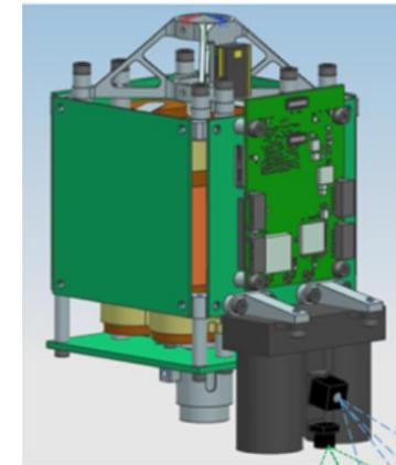
NASA Mars Helicopter Scout, sensor assembly. Monocular vision setup (2° camera only for sporadic hi-res images, not used for navigation) [1]
