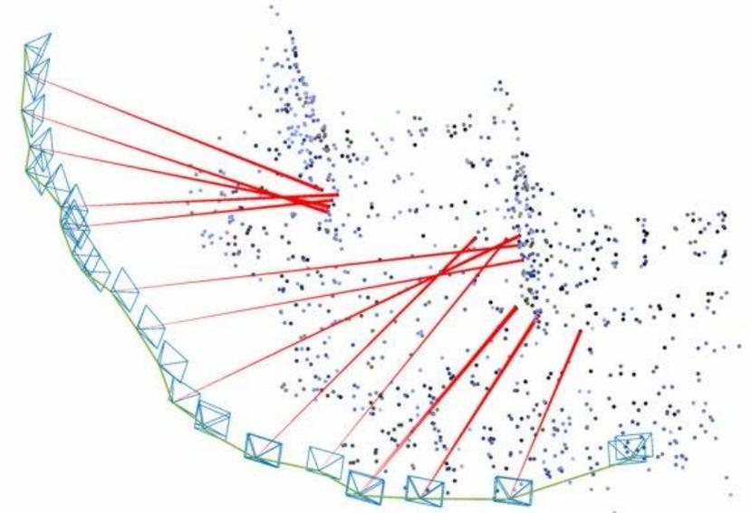
Camera poses, 3D landmarks and range measurements in a correctly scaled monocular reconstruction [3]
