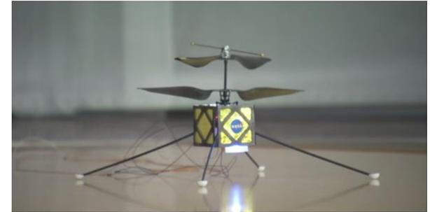
NASA Mars Helicopter Scout: first *soon-to-fly* planetary aerial explorer
