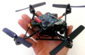
Monocular Visual Odometry aided by a Low Resolution Time of Flight Camera (8x8 pixels @ 20Hz):
