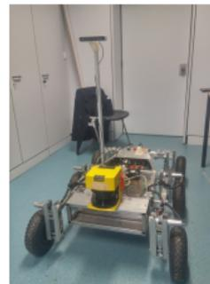
MORPHEUS rover with LiDAR and stereo camera
