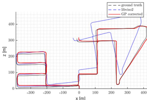
**Figure:** Blue line is LibVISO2 raw estimate. Red line is LibVISO2 corrected estimate from the error predictions. Black line is the DGPS reference trajectory
