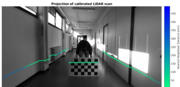
Calibration of the lidar-camera extrinsics
