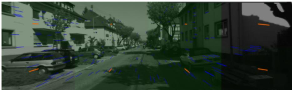
**Figure:** Green shade: feature density. Red lines: direction of the mean optical flow. Image from KITTI automotive benchmark
