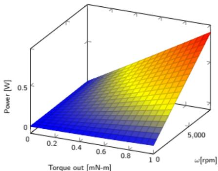
Figure: Electrical power required given  $T$  and  $\omega$
