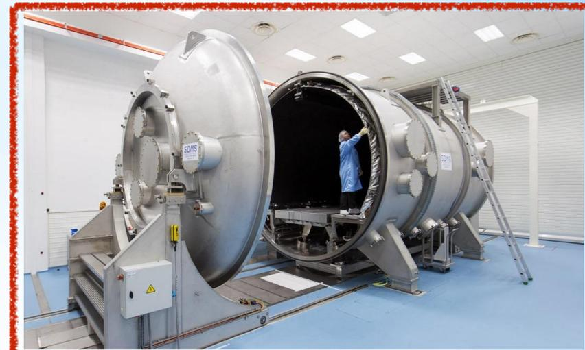
45 m<sup>3</sup> cryo-vacuum chamber
