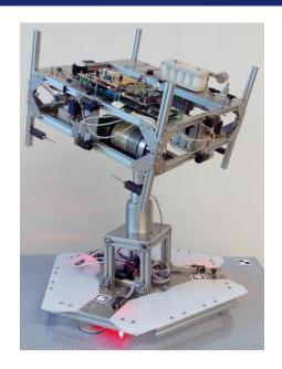
SPARTANS: cooperating SPAcecRaft Testbed for Autonomous proximity operatioNs experimentS
