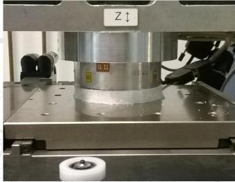
EPS Compressive Stress-Strain [Ro=17 Kg/m^3]
