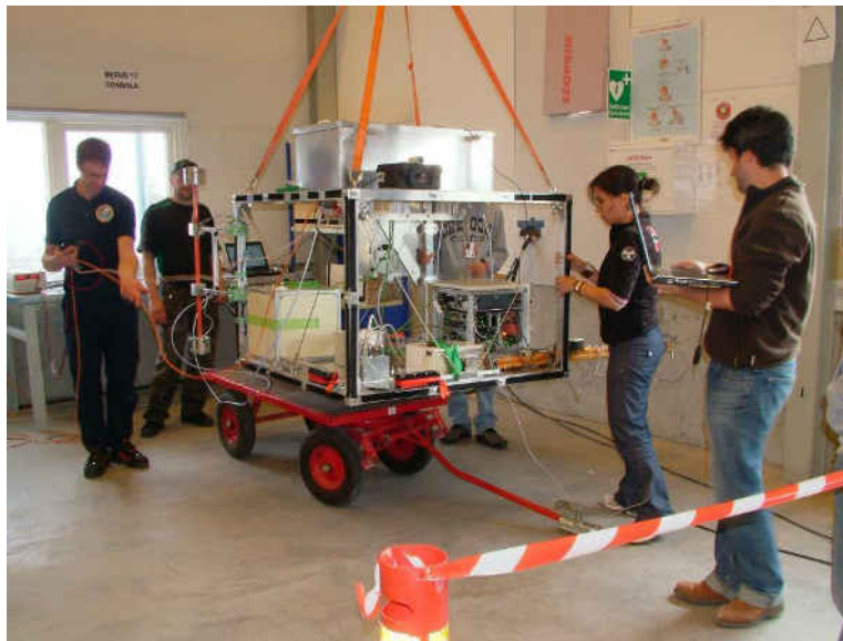
Rotation of the gondola needed for magnetometer calibration
