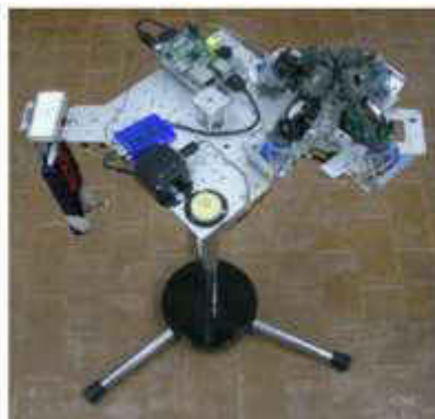
S5Lab 3 DoF ADCS test-bed equipped with Control Moment Gyros (CMGs)
