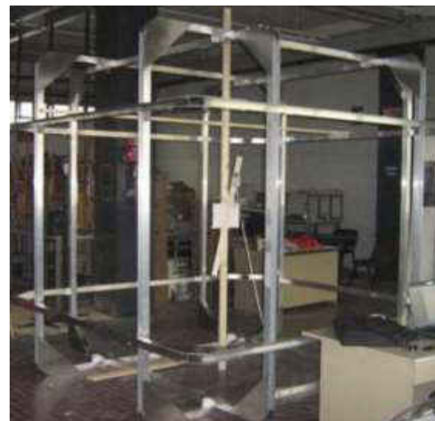
S5Lab 3D Helmholtz coil system (Magnetic field simulator)
