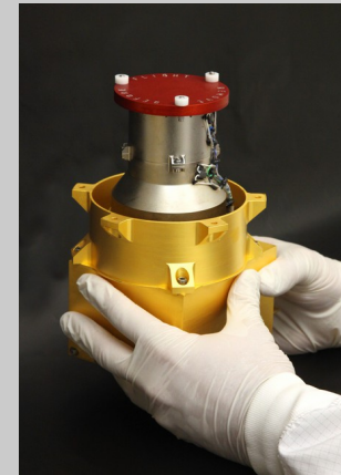
RAD "Radiations Assessment Detector", 1.5Kg © NASA
