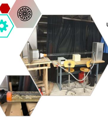
A preliminary test bench has been designed to simulate the working condition. The first goal is to understand the flow regime inside the pipe, hence the right measurement technology can be found. Once perfected, the bench will be used to test the different solution found
