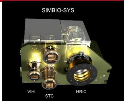
STC main scientific objective is the global mapping of the entire surface of Mercury in 3D.
