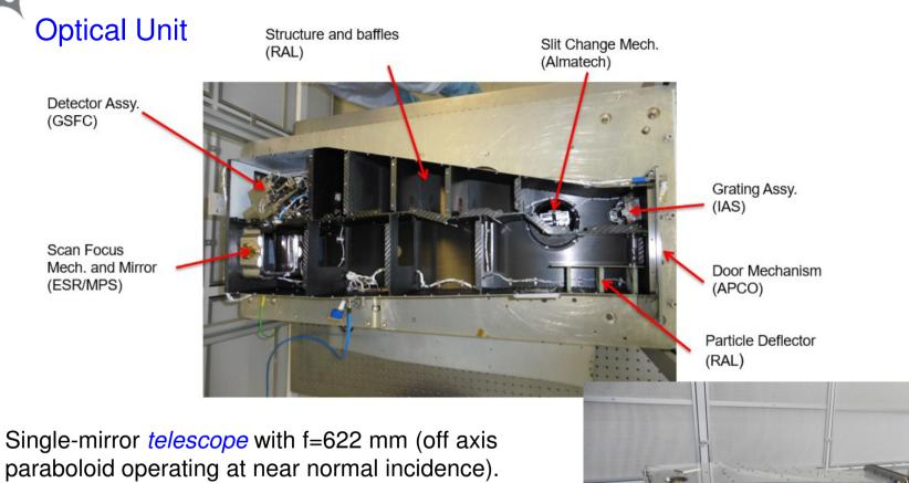
A Toroidal Variable Line Space *grating* images a choice of 4 spectrometer slits.
