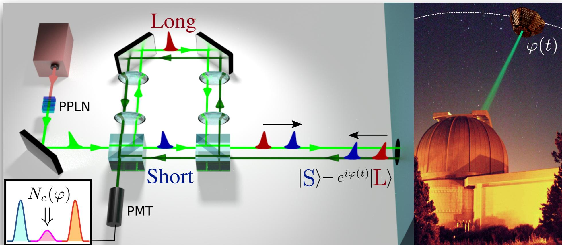
Two short pulses of light delayed by few nanoseconds are sent to the satellite which bounces them back to Earth where they are collected at the single-photon level because of the long journey. At the reflection the satellite introduces a phase-shift between the two pulses, due to its relative velocity respect to the ground station. When the photons are temporally recombined at the ground station, they interfere accordingly to the modulation imposed by the satellite motion.
