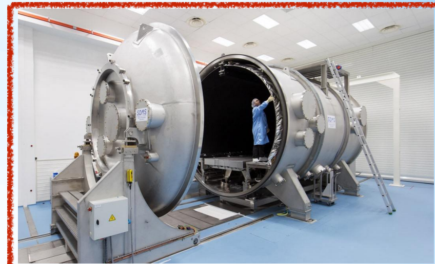
45 m 3 cryo-vacuum chamber 77K and 10 -6 mbar Large integration room (100tn seismic mass to provide high stability (< 10 -7 g at 5 - 100 Hz))
